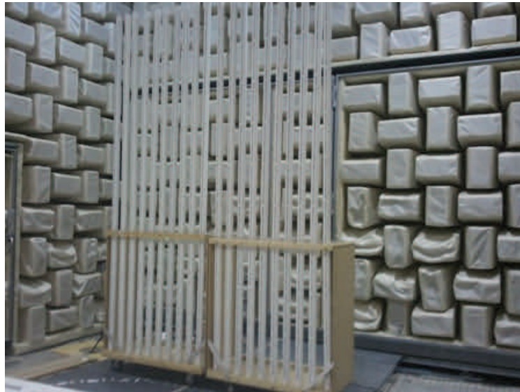
Experimental set-up in the anechoic chamber facilities in the Department of Aeronautical and Automotive Engineering to ensure free field conditions, and that the results are reliable
